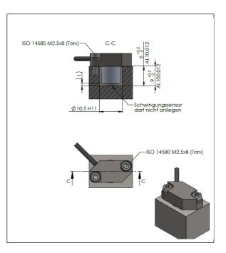
mounting with screws ISO 14580 (Torx) or DIN 7985-M2.5x8: (cylindric part of sensor must not touch machine housing)
